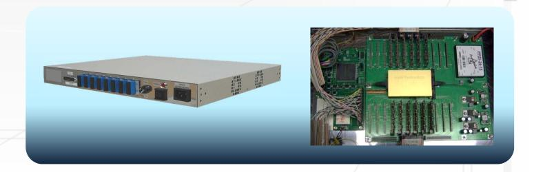
The PLZT Ultra-high Speed Optical Switching System with an internal FPGA controller enables high-speed optical switching networks easily and quickly.
